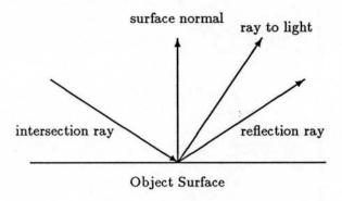
Using the rays shown above and the object's surface properties, the color of the point being shaded is determined.
