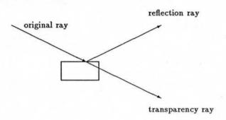
A reflection ray is sent from the point being shaded by a call to intersect. intersect finds the closest intersection with another object. Then it calls shade to determine the color at the point of intersection and returns the color. This color is combined with the color already calculated for the point being shaded.
