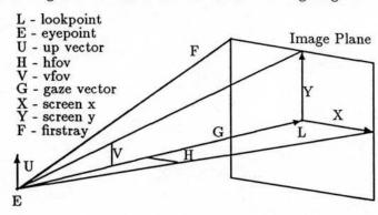
The eyepoint (E) describes the camera position. The lookpoint (L) describes where the camera is pointing. It is the center of the image plane. Together, the eyepoint and the lookpoint define the gaze vector (G). The up vector (U) describes the orientation of the camera about the gaze vector.
