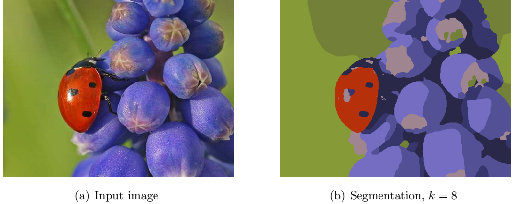
Figure 16: Piecewise constant Mumford-Shah segmentation of a natural image. (a) shows the input image and (b) is the minimizer of energy (89). The mean color values c_i of the partitions have been initialized using k-means clustering.
