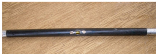
Fig. 7 The shaft model with glued strain gauges
