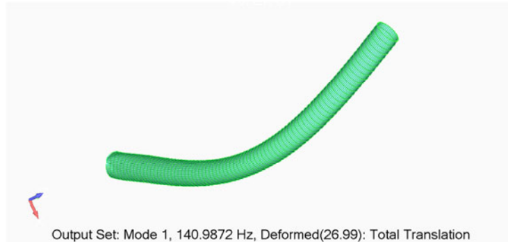
Fig. 5 Fundamental natural frequency of the hybrid Al/USN150 carbon fibre/epoxy composite shaft
