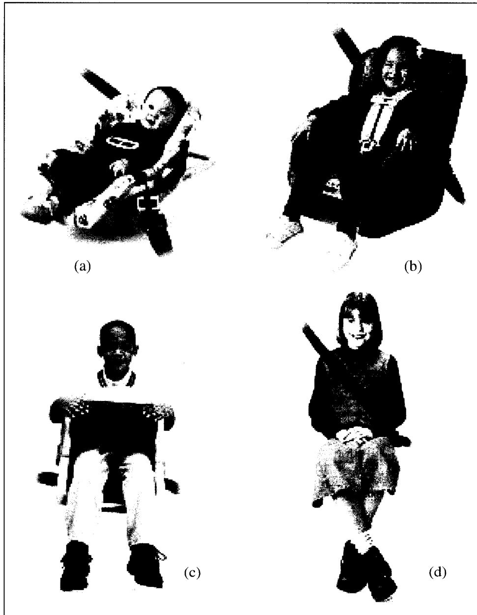
Figure 1. Suggested modes of restraint for various ages and sizes of children: (a) rear facing car seat, (b) convertible child safety seat, (c) booster seat with a shield booster is used when only lap belts are available, and (d) child weighing 36 kg or over eight years of age should fit properly in adult restraints [16].
