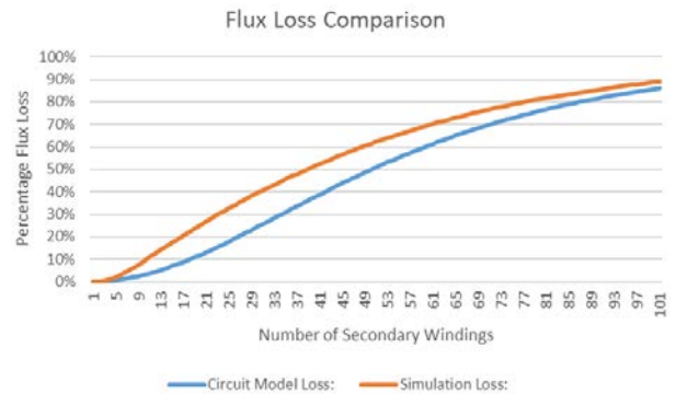
Fig. 10. The maximum loss of flux linkage in clamped return path ICTs with an incrementally increasing number of secondary windings, predicted using both the flux circuit model and FEA.
