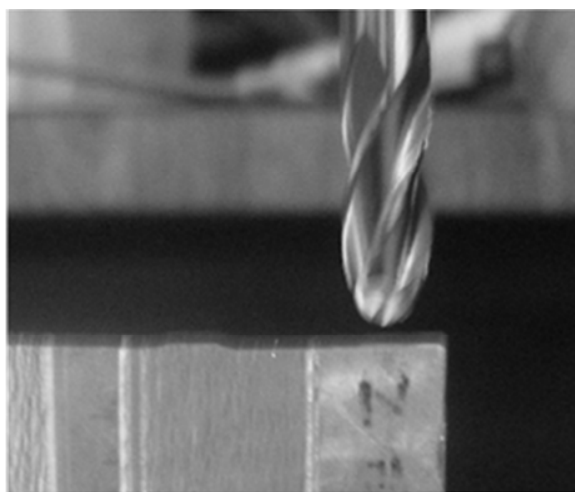
(b) Detail of ball nose end mill.
