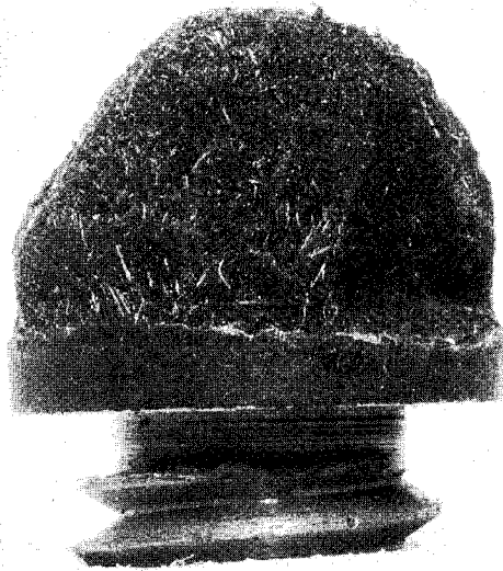
(a) Run 27; K = 0.00 ; p_{t,2} \approx 5.2 atm; run time 2 sec; H_0 = 3.11 kg/m 2 -sec.
