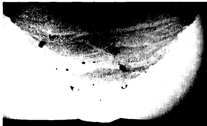
C. Test Weld No. 20 Total Acoustic Emission 411
