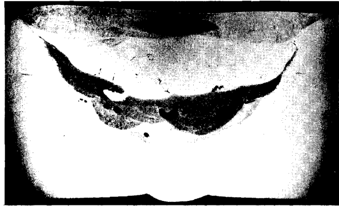
A. Test Weld No. 7 Total Acoustic Emission 426
