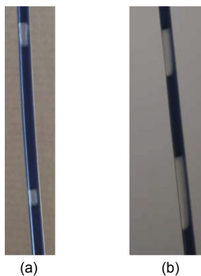
Fig. 3 Bubbles in 4.0 mm PU hoses (a) Bubbles in upper hose; (b) Bubbles in lower hose
