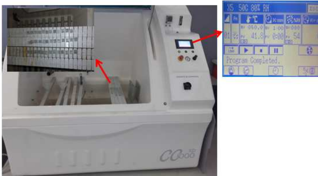
(b) Adhesively bonded composite samples and hygrothermal aging conditions
