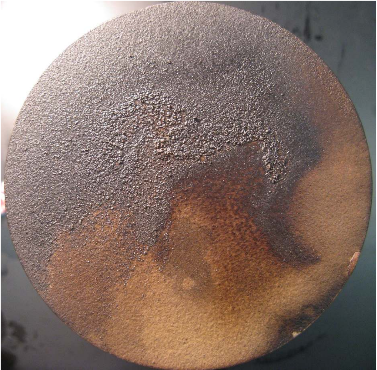
Figure D.3: YSZ coated piston crown after testing
