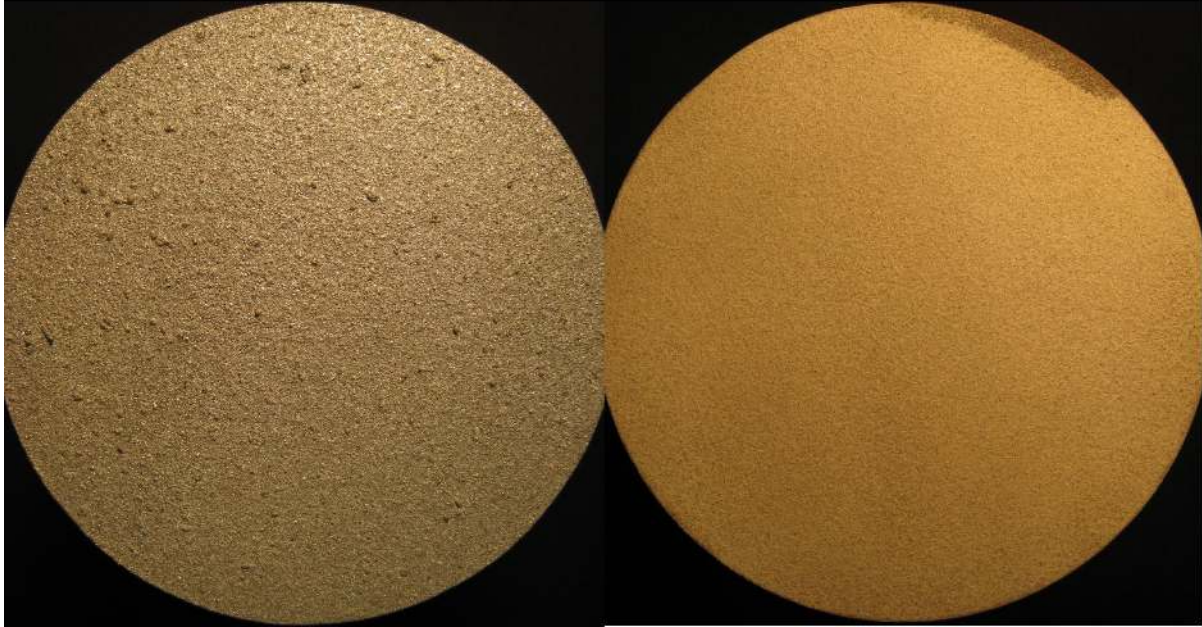
Figure 6.7: Pictures of TBCs prior to testing (left - metal TBC, right - YSZ)
