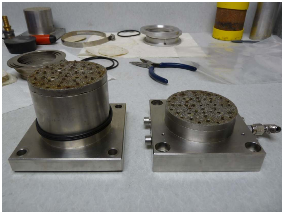
Figure 3.11: End platens of the DCSS.
