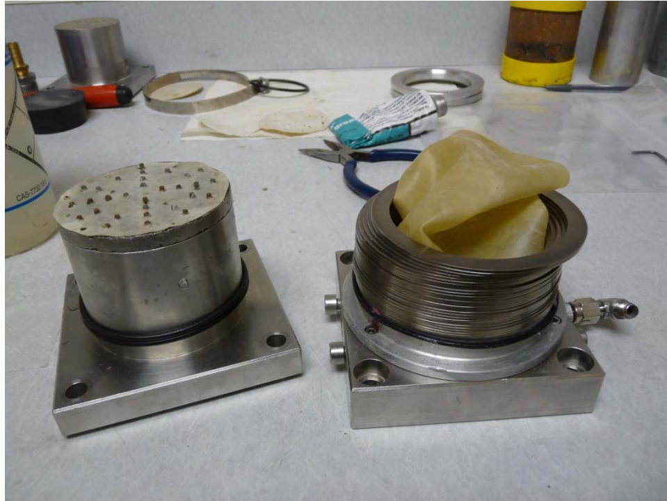
Figure 3.12: End platens with filter paper, metal ring, membrane and Teflon coated rings.
