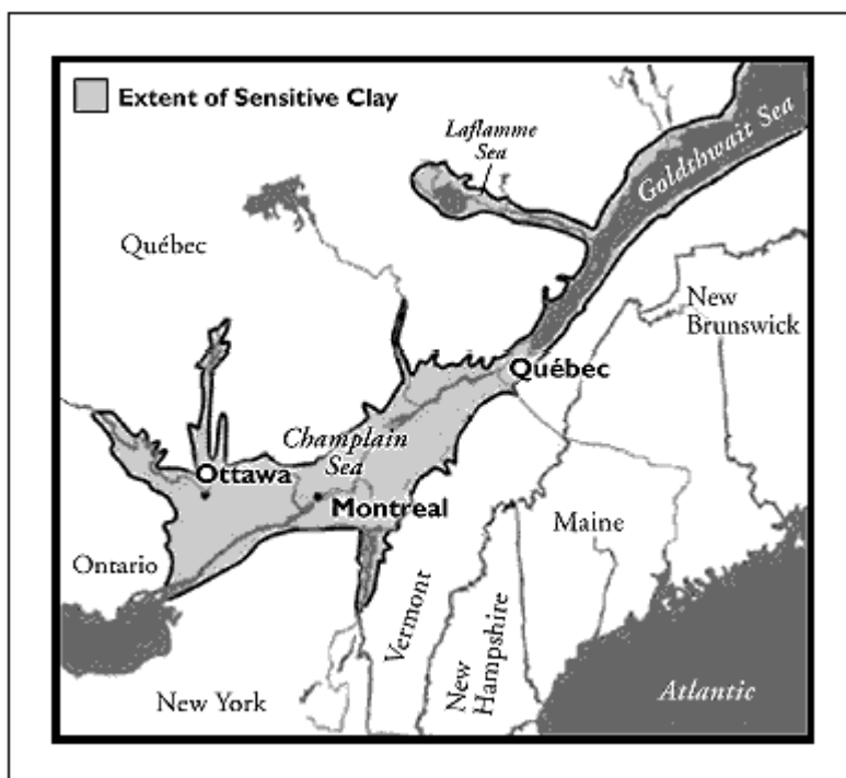
Figure 2.1: Extent of sensitive clay in Eastern Canada (Canadian Mortgage and Housing Corporation, 2001).
