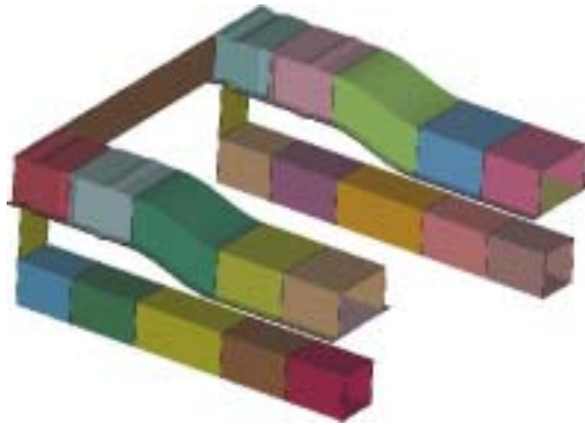
Figure 2 Front rail structure
