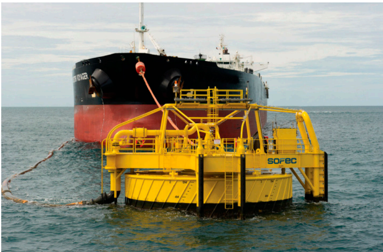
Figure 2. CALM Buoy attached to an FSO in the Baltic Sea offshore Lithuania (Adapted with permission of SOFEC Inc.; Courtesy: SOFEC; Source: [49]).
