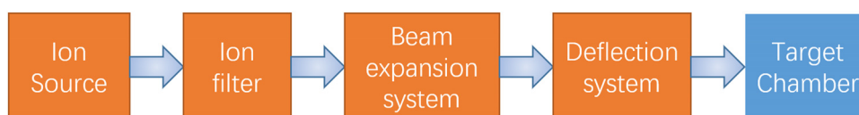
Figure 1: The schematic diagram of an ion beam system.
