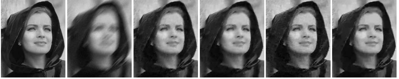
Figure 5. Deconvolution example with known blur kernel. Shown is a zoom to the right face part of romy. From left to right: Original image, degraded image with motion blur of length 30 rotated by 45^\circ and Gaussian noise with \sigma = 5 . Deconvolution using TGV with \lambda = 400 , \alpha_1 = 0.5 , \alpha_2 = 1.0 ( PSNR = 29.92 ), non-convex log-TGV, \beta = 1 , with \lambda = 300 , \alpha_1 = 0.5 , \alpha_2 = 1.0 ( PSNR = 30.15 ), the learned prior [15] with \lambda = 25 ( PSNR = 29.71 ), and its non-convex counterpart with p = 1/2 and \lambda = 40 ( PSNR = 30.54 ).
