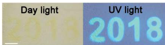
Fig. 5 Photographic images of 2 in PEO. The letters were generated upon irradiation at 365 nm. The scale bar is 2 mm.
