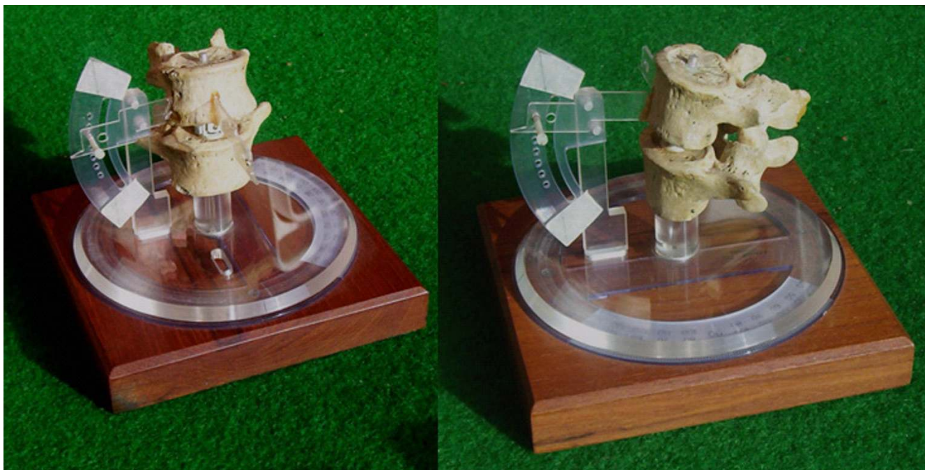
Figure 4 Calibration model I. with inter-body universal joint and calibrated protractors for intervertebral angle and whole model rotational settings
