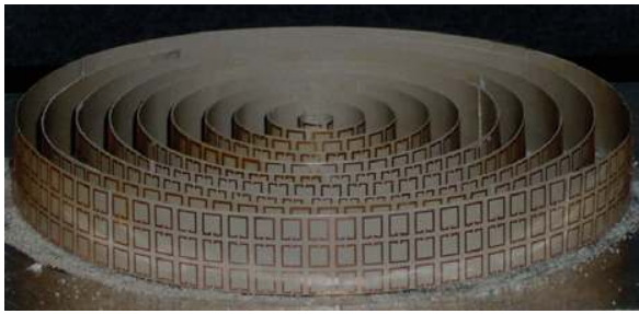
Figure 3 | The device. The split-ring resonators constitute a metamaterial for microwave radiation with the designed radial magnetic permeability (6). The rings were then filled with a white dielectric powder that generates the required electric permittivity of n_0^2 (not shown here).
