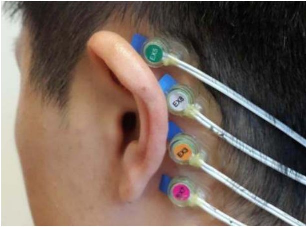
Fig. 7. Placements of four behind-the-ear electrodes while subjects performed the online SSVEP experiment.
