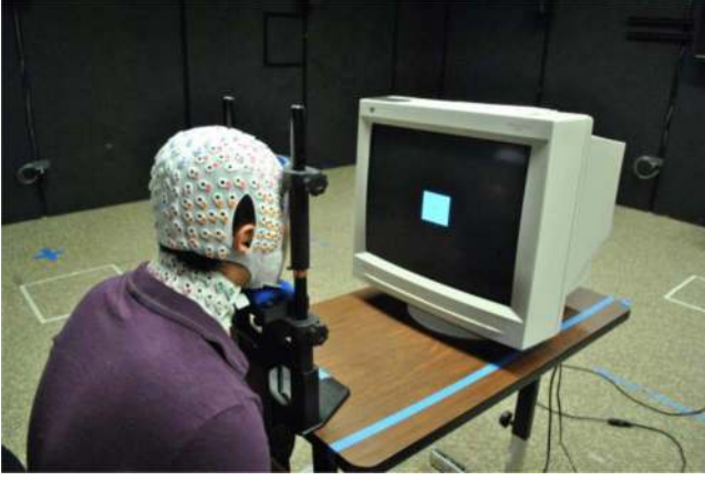
Fig. 1. Subject wore a 256-channel EEG recording system (includes a cap and a neck band) and gazed at a visual stimulus with his head resting on a chin rest. Note that all the cables were removed temporarily in order to have a clean view.
