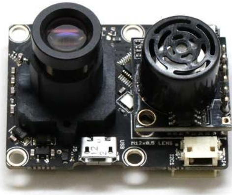
Fig. 1. The presented PX4FLOW optical flow sensor with mounted lens on the left and ultra sonic distance sensor on the right.
