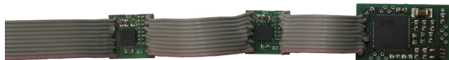
Fig. 4: The version of the MIMU platform where the IMUs are mounted on separate boards, which are connected in a daisy chain to the \mu\text{C} board.
