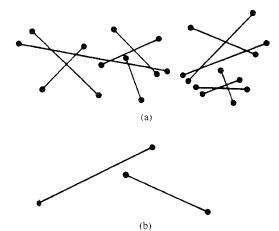
Fig. 7. (a) Twelve segments that satisfy the clearance property. (b) It takes only two segments to violate the clearance property.
