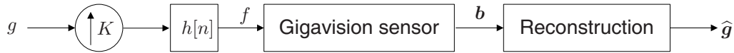
Figure 4. The equivalent model for the gigavision camera. g = [g[1], g[2], \dots, g[M]]^T is critically sampled light intensity values. K = \frac{N}{M} is the upsampling factor. h[n] is a low-pass filter. f = [f[1], f[2], \dots, f[N]]^T is the oversampled light intensity values. \mathbf{b} = [\mathbf{b}[1], \mathbf{b}[2], \dots, \mathbf{b}[N]]^T is the binary image. \hat{\mathbf{g}} = [\hat{\mathbf{g}}[1], \hat{\mathbf{g}}[2], \dots, \hat{\mathbf{g}}[M]]^T is the reconstructed light intensity values.
