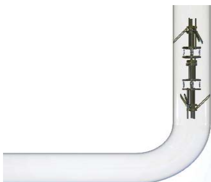
(e) Clamped legs and retracted central module, vertical position of robot
