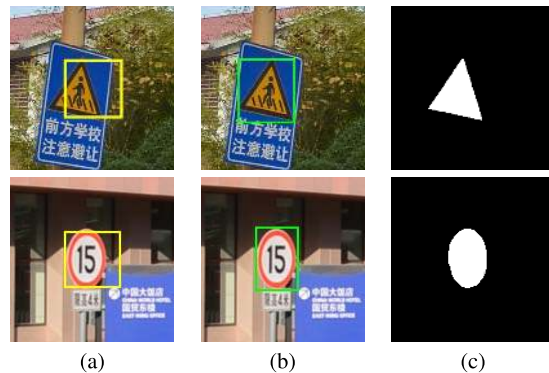
Fig. 1. Two examples of traffic sign localization: (a) Detection result using a cascaded detector (yellow rectangle). (b) Optimized detection result using our approach (green rectangle). (c) Segmentation result (white pixels).
