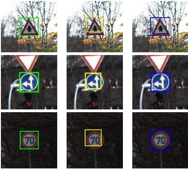
Fig. 5. Localization refinement results for examples from GTSDDB. Rows: different categories of sign. Left: after refinement by our approach. Center: output of standard detector. Right: ground truth annotation.
