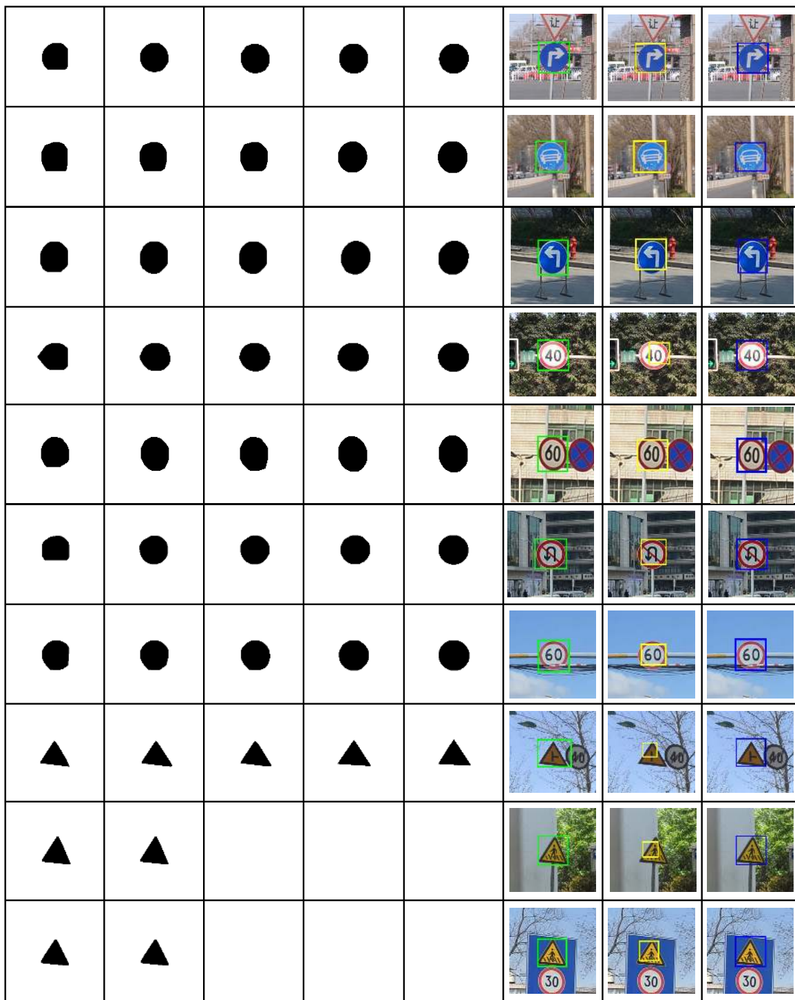
Fig. 9. Detection refinement results for various CTSDB images. Columns 1–5: segmentation results as iteration proceeds. Column 6: our localization results (green rectangles). Column 7: unrefined input from the cascade detector (yellow rectangles). Column 8: ground truth annotations (blue rectangles).
