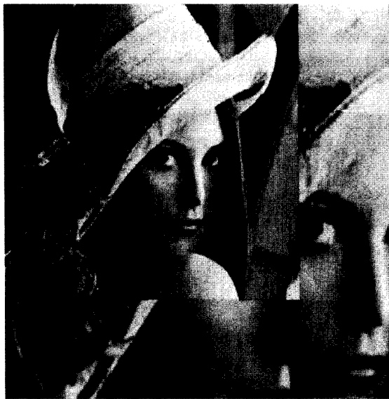
Fig. 4. In this picture anisotropic low-pass filtering is applied to boundary pixels in the JPEG quantized image shown in Fig. 2. We still notice the remaining blocking effects around the cheek area.
