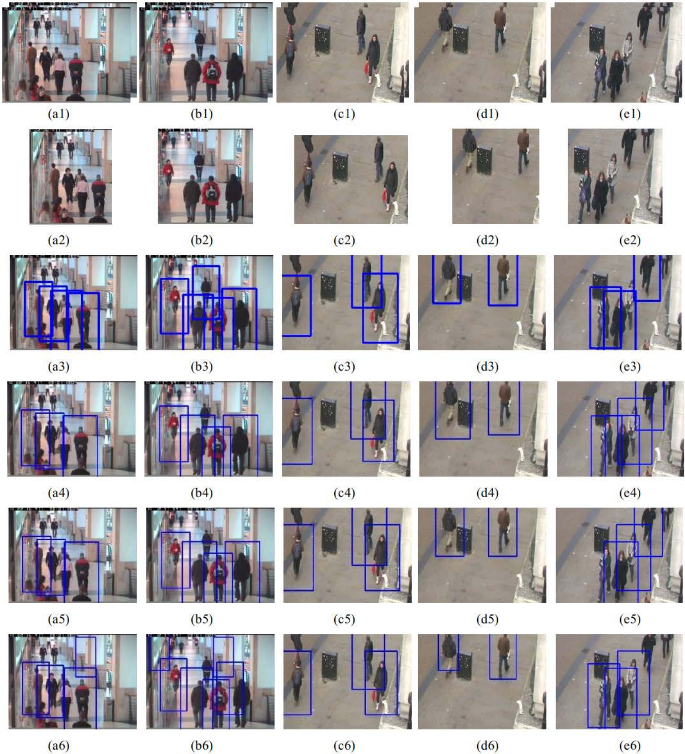
Fig. 8. Video Images (a1-e1), ROI (a2-e2), Results of original HOG (a3-d3), SW3S (a4-d4), SW2S (a5-d5), DW3S (a6-d6)
