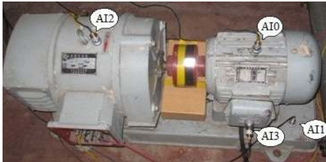
Fig. 7. Positions of acceleration sensors
