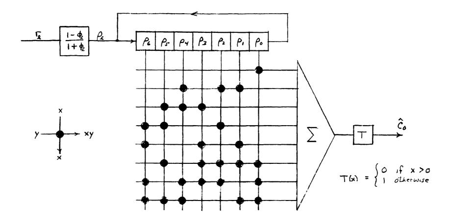
Figure 1. Decoder for the (7,4) code.
