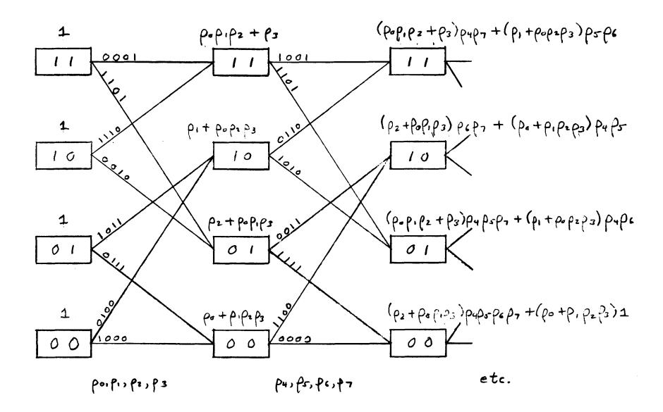
Figure 2. Decoder for the (4,3,3) code.
