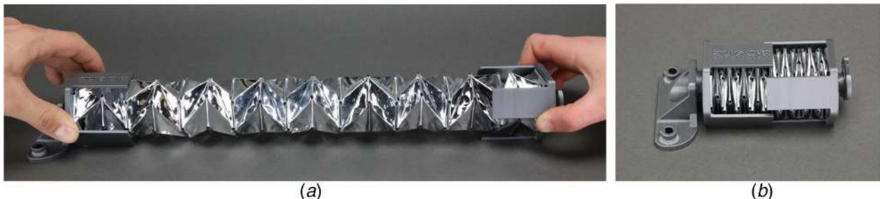
Fig. 13 Metallic-backed PET OriGuide. (a) Extended and (b) compressed.
