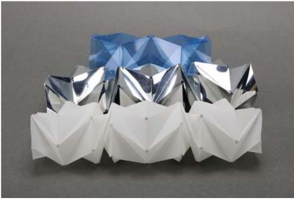
Fig. 11 Pattern demonstrated in matte, colored, and reflective, metallic-backed PET
