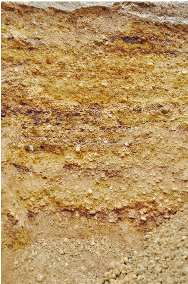
Fig. 8: Outcrop of the Federnberg Schotter (location south of Ried/Innkreis, see Fig. 5) showing horizontally bedded and oxidized gravel with rounded clasts consisting predominantly of quartz and quartzite (outcrop height is approximately 2 m). Layers of clast-supported gravel with open-framework are indicative for deposition by braided river.
