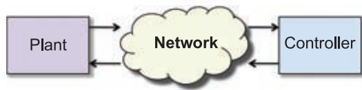
Figure 5: Structure of networked control systems.
