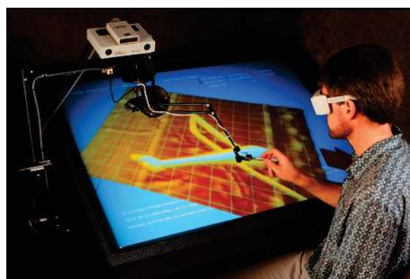
(a) NanoManipulator application: virtual microscope. Image courtesy of the UNC Computer-Integrated Systems for Microscopy and Manipulation NIH 5-P41-RR02170-21
