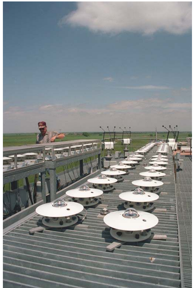
Fig. (2). Radiometers on a Radiometer Calibration Facility deck located near Lamont, Oklahoma.
