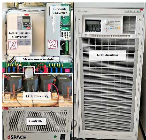
Fig. 14. Laboratory setup used to validate the reviewed methods. The line-side converter is regulated using a dSPACE control platform to inject currents through an LCL filter into a grid simulator.
