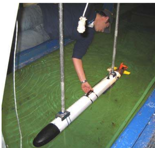
Figure 9. Vehicle testing at MHL tow tank.
