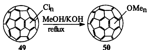
Figure 18. Replacement of chlorine atoms by methoxy groups.
