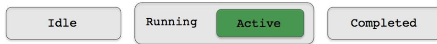
Figure 14: Behavior States: A behavior may be in one of these four states at any given iteration of helm Iterate() loop. The state is determined by examination of MOOS variables stored locally in the helm’s information buffer.
