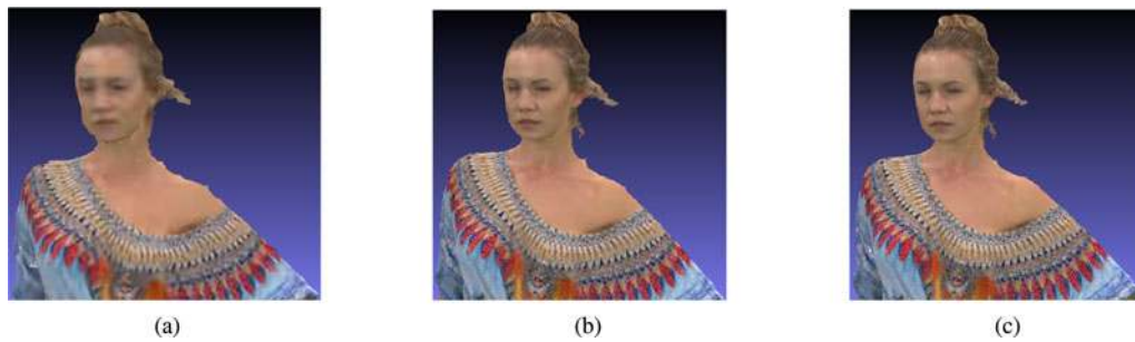
Fig. 19. Subjective quality using PCC Rendering Software, (a) Longdress at 2.2 Mbps, (b) Longdress at 10.9 Mbps, (c) Longdress at 25.2 Mbps.
