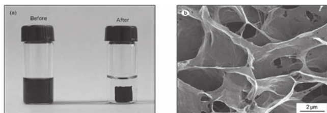
Figure 6. a) Photograph of an aqueous mixture of GO (2 mg/mL) and sodium ascorbate before (left) and after (right) chemical reduction. b) SEM image of AQSGH. Reproduced with permission. [87] Copyright 2010, American Chemical Society.
