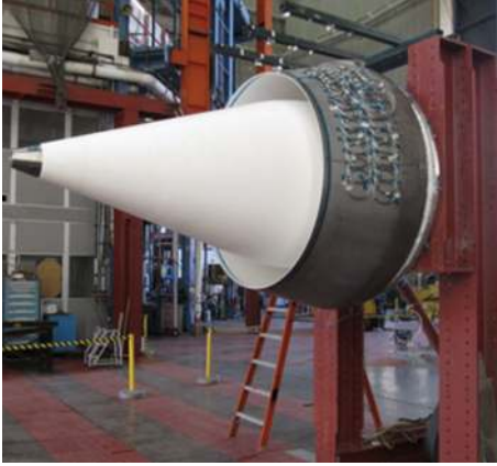
FIGURE 1: Oxide ceramic matrix composites exhaust ground test demonstrator consisting of a 1.60 m diameter nozzle (showing underneath the titanium-alloy faring) and 1.14 m diameter by 2.34 m conical centerbody with titanium end cap inspection portal (Courtesy of Wiley, Steyer [1]).
