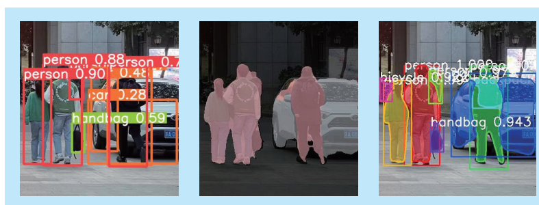
Figure 18. From left to right are the test renderers of YOLOv5, Deeplabv3, and Mask R-CNN.
