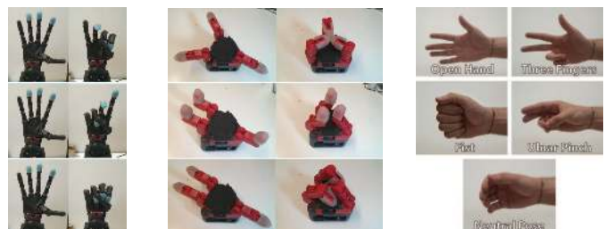
(a) Top to bottom: Tripodal, Ulnar and Power grasps. (b) Top to bottom: Tripodal, Parallel and Cylindrical grasps. (c) Gestures to be classified.
