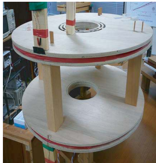
FIGURE 8: Three-coil pair system Helmholtz coil.
