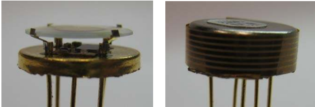
Figure 5-18: Miniaturizing an OCXO with a typical resonator by applying one-chip temperature control, flexible circuit, and ACF-bonding.
