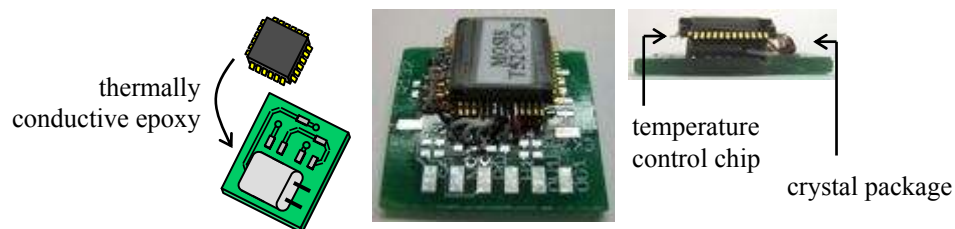
Figure 3-20: Low-cost OCXO structure with a quartz resonator in HC49/U and a packaged temperature-control chip.
