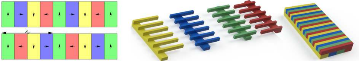
Figure 15. Rendering of a proposed undulator and assembly approach in the style of [96], showing a standard Halbach geometry with manufacturing techniques adapted to mm-period scale.
