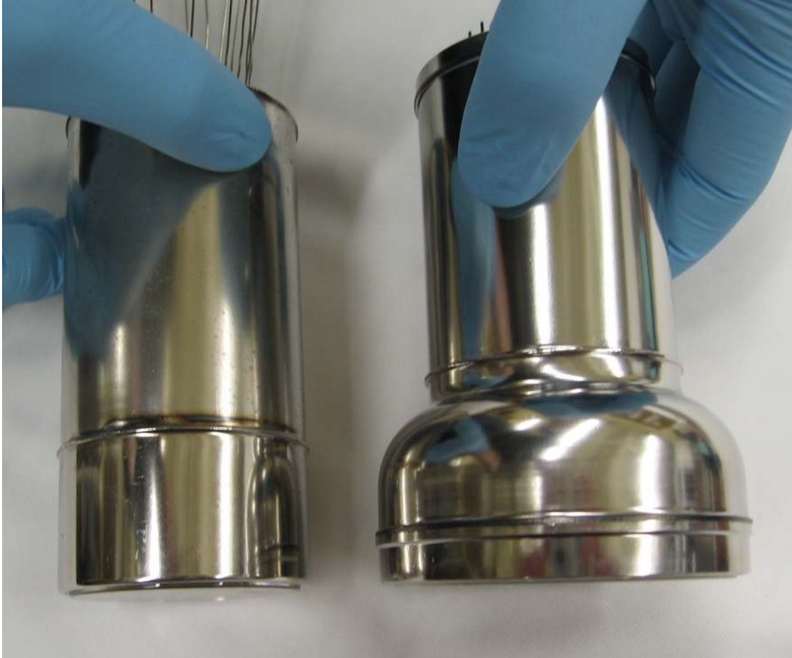
Figure 1: The Hamamatsu R8778 PMT, used in the LUX experiment (left), and the R11410 MOD PMT, a candidate for use in the LZ detector (right). The R11410 MOD features a 6.4 cm diameter photocathode, offering twice the surface area of the 4.5 cm diameter R8778 photocathode.
