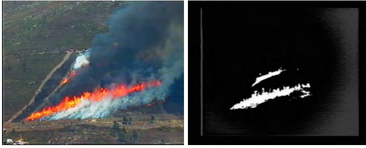
Fig. 8 A visual (left) and an infrared (right) images of the same fire at approximately the same time instant. Infrared images are not affected by smoke, and therefore they also provide negative information.
