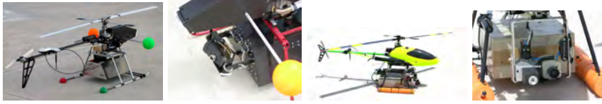
Fig. 3 The vehicles carry mainly IMUs and GPS for navigation. Also, cameras on pan and tilt units for perception.
