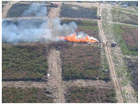
Fig. 12 An aerial view of some of the plots employed during the fire experiments at Gestosa, Portugal. The plot side in this case is around 75 m.
