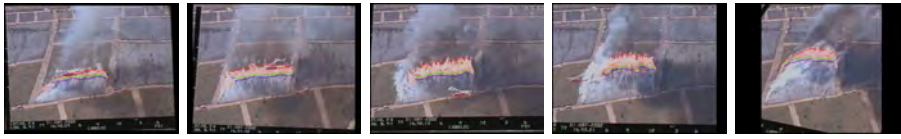
Fig. 13 Frames 3, 44, 77, 144 and 219 of the aerial sequence gathered during the fire experiment 520, after automatic stabilization. The extracted fire front contour is also shown.
