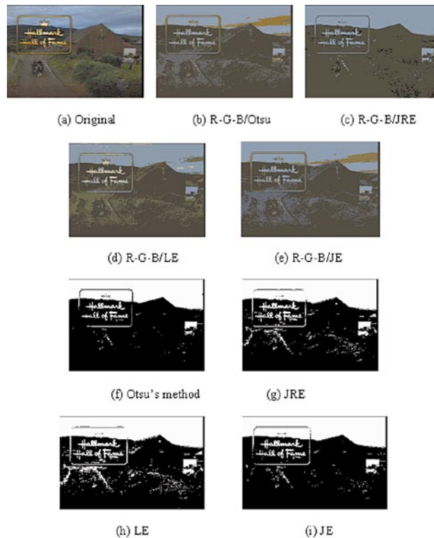
Fig. 7 A countryside scene: (a) original, (b) RGB/Otsu, (c) RGB/JRE, (d) RGB/LE, (e) RGB/JE, (f) Otsu's method, (g) JRE, (h) LE, and (i) JE.
